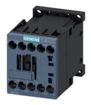
power contactor, AC-3e/AC-3, 9 A, 4 kW / 400 V, 3-pole, 220 V AC, 50 Hz / 240 V, 60 Hz, auxiliary contacts: 1 NC, screw terminal, size: S00
