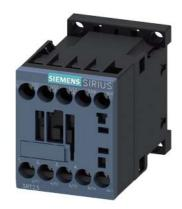
contactor AC-1, 18 A, 400 V / 40 °C, 4-pole, 24 V DC, screw terminal, size: S00  $\,$
