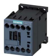
power contactor, AC-3e/AC-3, 9 A, 4 kW / 400 V, 3-pole, 200 V AC, 50 Hz / 200-220 V, 60 Hz, auxiliary contacts: 1 NO, screw terminal, size: S00
