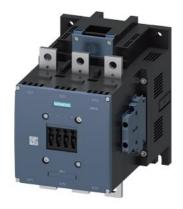
power contactor, AC-3e/AC-3 500 A, 250 kW / 400 V AC (50-60 Hz) / DC Uc: 110-127 V 3-pole, auxiliary contacts 2 NO + 2 NC drive: conventional main circuit: busbar control and auxiliary circuit: screw terminal
