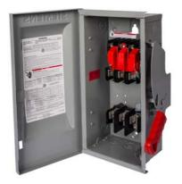
Siemens Low Voltage Circuit Protection Heavy Duty Safety Switches. Type: ENCLOSED, SAFETY SWITCH Std: UL V. Rating: 600V A. Rating: 200A Wattage: 4W No. Of Poles: 3P F. Rating: 60Hz Action: SINGLE THROW Material: 304SS Enclosure: TYPE 3R. 2-3 point mounting holes. O. Cycles: 8000 O. Temperature: (-20F-120F) AMBIENT TEMPERATURE Environmental Conditions: OUTDOOR
