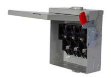
Siemens Low Voltage Circuit Protection General Duty Safety Switch. 2-Pole 2-Fuse and solid neutral Fused in a type 3R enclosure (outdoor). Rated 240VAC (100A). Horse power (Std, Time delay) fused: 1-PH 2-W (7-1/2, 15), 3-PH 3-W (15, 30), 250VDC (20). Special features: service entrance labeled suitable for 3-PH motor loads
