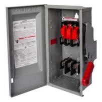
Siemens Low Voltage Circuit Protection Heavy Duty Safety Switches. Type: ENCLOSED, SAFETY SWITCH Std: UL V. Rating: 600V A. Rating: 100A Wattage: 3W No. Of Poles: 3P F. Rating: 60Hz Action: SINGLE THROW Material: 304SS Enclosure: TYPE 3R. 2-3 point mounting holes. O. Cycles: 10000 O. Temperature: (-20F-120F) AMBIENT TEMPERATURE Environmental Conditions: OUTDOOR
