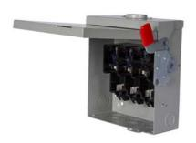
Siemens Low Voltage Circuit Protection General Duty Safety Switch. 2-Pole 2-Fuse and solid neutral Fused in a type 1 enclosure (indoor). Rated 240VAC (200A). Horse power (Std, Time delay) fused: 1-PH 2-W (15, -), 3-PH 3-W (25, 60), 250VDC (40). Special features: service entrance labeled suitable for 3-PH motor loads.
