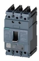
circuit breaker 3VA5 UL frame 125 breaking capacity class S 25kA @ 480V 3-pole, line protection TM230, FTAM, In=20A overload protection Ir=20A fixed short-circuit protection Ii=7.5...15 x In without connection
