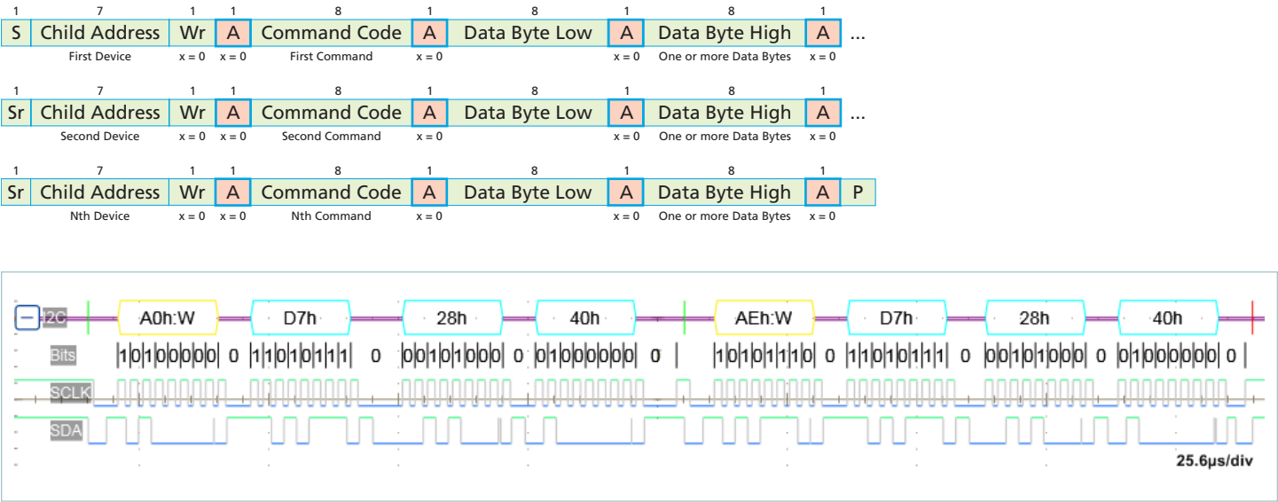
Figure 7 — DISABLE_FAULT COMMAND (D7h)_WRITE
