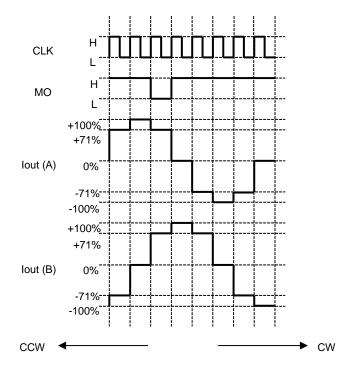
Note: MO signal is shown in the above timing chart when MO pin is connected with a pull-up resistor to VCC. Note: Timing charts may be simplified for explanatory purpose.
