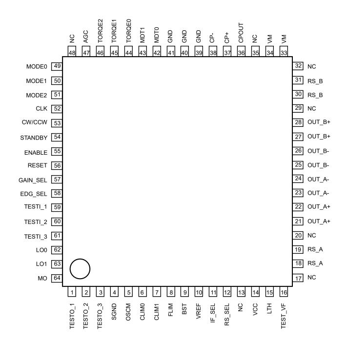
Note: Please solder the corner pads and the rear thermal pad of the QFN package, to the GND pattern of the PCB.
